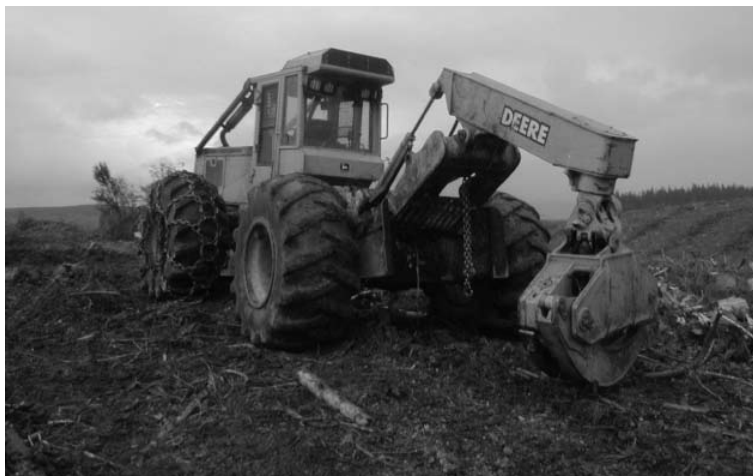
Figure 2. The soil at the site was trafficked by two rubber tyred skidders and one forwarder. Photo: Matt Wood
